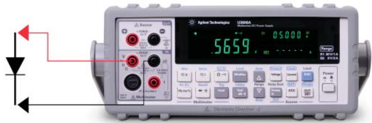
Figure 1. Forward-biased condition in a diode
