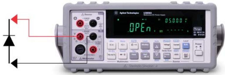
Figure 2. Reverse-biased condition in a diode
