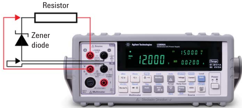
Figure 5. Zener diode test using the U3606A
